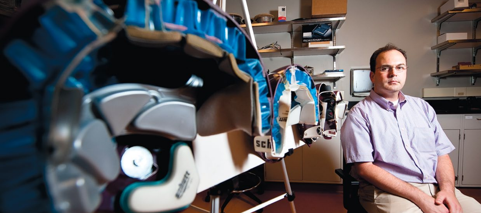
A line of football helmets cut in half shows pads and sensors on each different model or manufacturer style.
