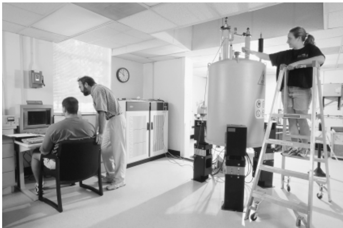
Professor of Chemistry Mark Welker (standing, left) and students with the 500 MHz NMR spectrometer.
