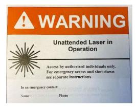
Temporary Laser Controlled Areas for Class 3B and Class 4 laser systems must have appropriate NOTICE signs. Example:
