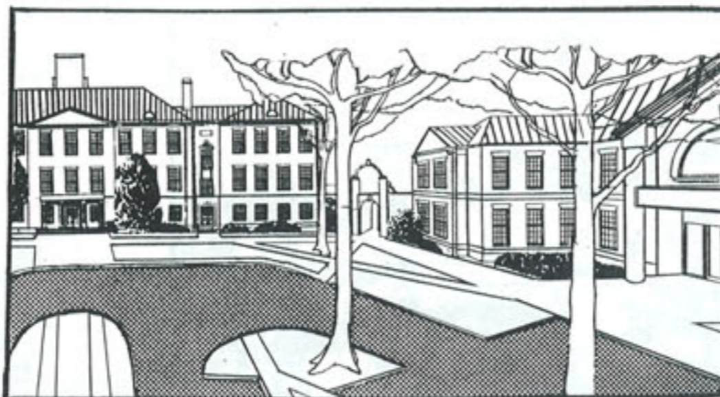
Fig. 11 Schematic representation to show relationship of proposed University Center building to western end of Reynolda Hall. The connecting arch detail matches details of the archway between Reynolda Hall and Davis House.
